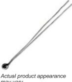
192 Series, Uni-Curve with bare leads and epoxy, 5,000 Ohm resistance, ±0,2 °C [0.36 °F] tolerance, 25/85 BETA = 3974
